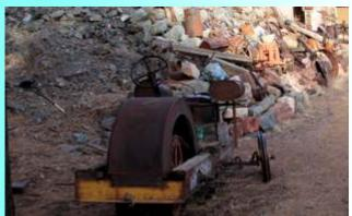
This s a Ford Model-T converted to a tractor. Farmers would buy a kit and convert the car to a tractor.
